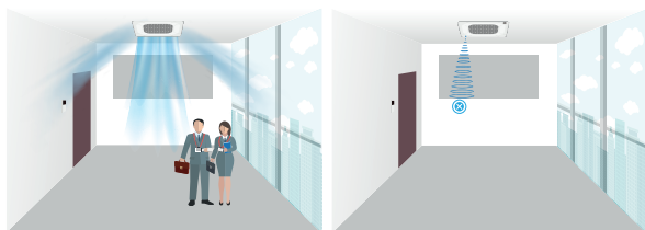
The indoor unit automatically runs when detecting human body
